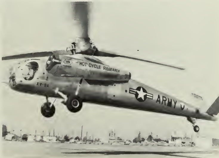
HOT CYCLE research helicopter now under development gets power from hot gases jetted through tips of rotor blades.
